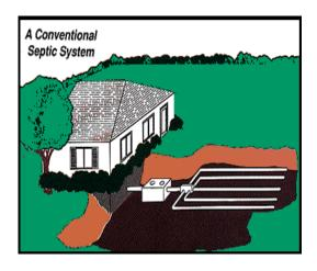
A typical septic system consists of a septic tank, a distribution box, and a drain field - all connected by pipes called conveyance lines.
