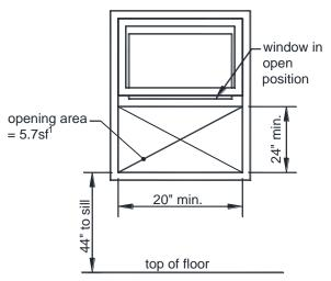
windows shall have a minimum net clear opening of 3.3 square feet. The minimum net clear opening dimensions shall be 20 inches by 24 inches in either direction.
