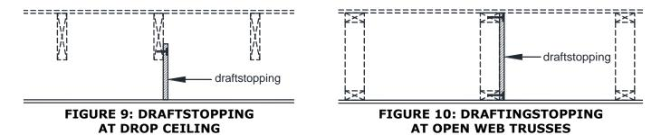
**Draftstopping material.** Draftstopping shall consist of ½-inch minimum gypsum board, ¾-inch minimum wood plywood/OSB or ¾-inch minimum particleboard, Type 2-M-W.
