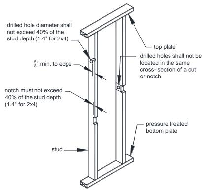
FIGURE 7: DRILLING AND NOTCHING STUDS
