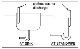
FIGURE 11: AIRBREAK AT CLOTHES WASHER DISCHARGE
